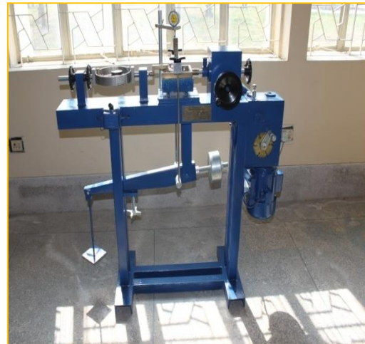
Direct Shear Test Apparatus
