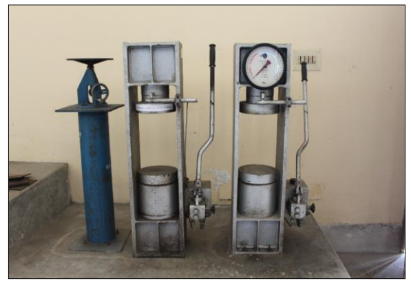
Compressive strength testing machine used for testing of concrete cylinder, block etc.
