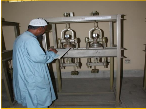
Consolidation Test Apparatus
