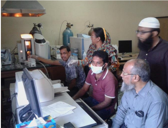
Heavy metals such as Zn, Al, Pb, B, Cd, Cr, Mg, Fe, As, Hg etc. of water samples are being detected by Atomic Absorption
