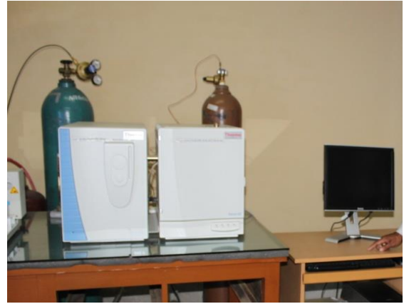
Gas Chromatography-Mass Spectroscopy to detect volatile organic compound in soil and water.
