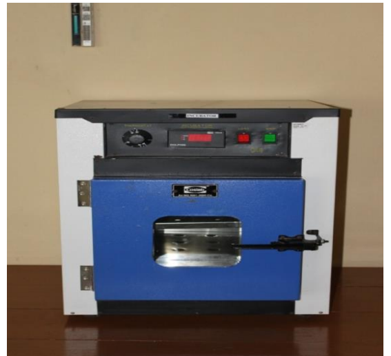
Incubator used to maintain required temperature of reagents and samples.
