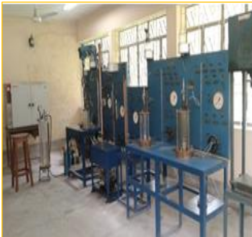
Triaxial Shear Test Apparatus
