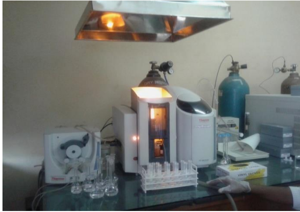
Heavy metals of soil samples detected by Atomic Absorption Spectrometer.
