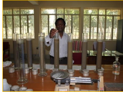
Equipment for Hydrometer Analysis
